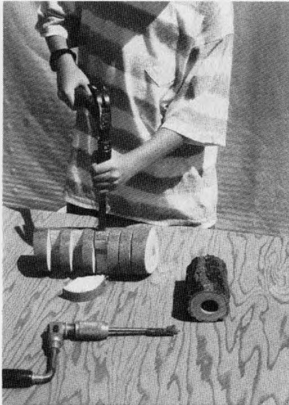
Above, Left: Why buy when you can make a rustic desk set that looks this good? Above: After making saw cuts, chip out the letter-holder "slices" with a hammer and chisel. A hand drill makes a clean hole in the pencil holder.
